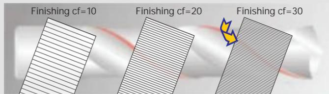
The 11V9 Wheel while grinding the OD, leaves grinding signs perpendicular to the work direction commonly called pitch. Closer the pitch finer the finish. The formula governing Surface Finish on OD of rotary tools is.
